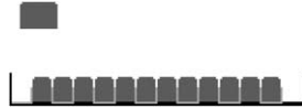
Fig. 1. Fragmented linear primary storage (feeder); insertion of a 2 slots wide item (component).
