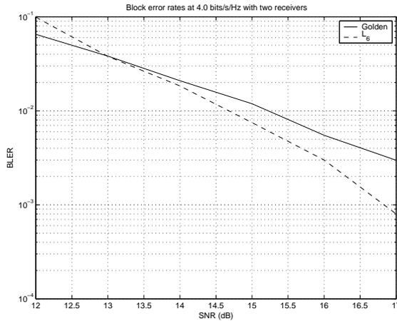
Figure 2: Block error rates at 4.0 bits/s/Hz with two receivers
