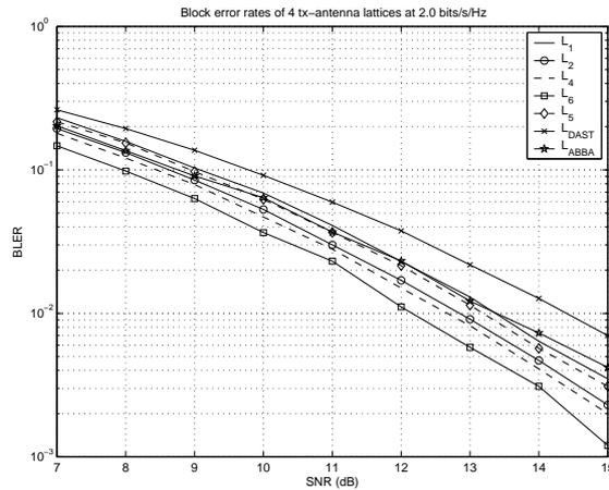
Figure 1: Block error rates of 4 tx-antenna lattices at 2.0 bits/s/Hz
