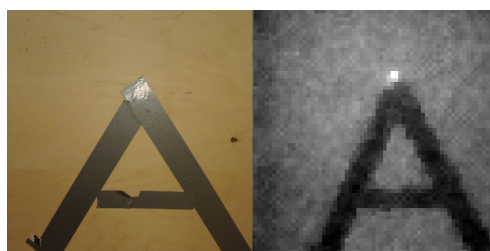
Figure 7: A “regular” digital camera and single-pixel camera photo side by side depicting an A figure.
