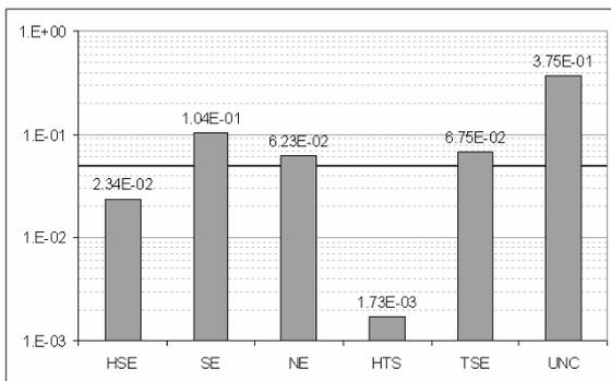
Figure 9. Ratio of visible erroneous seconds,  $C/N = 13$  dB,  $f_D = 30$  Hz (MFER SE  $\approx 10\%$ ).
