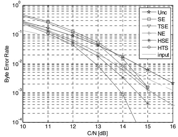
Figure 6. Byte Error Rate for Doppler frequency 10 Hz
