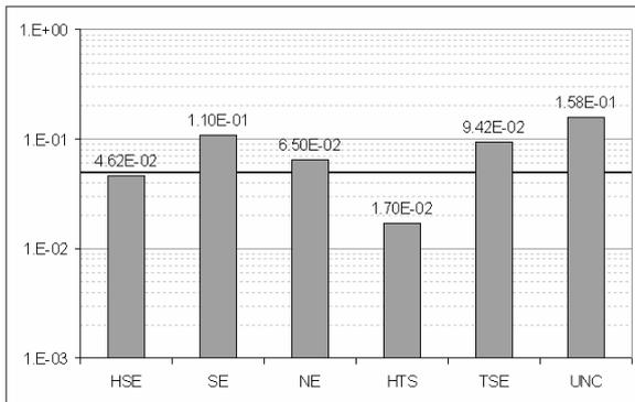
Figure 7. Ratio of visible erroneous seconds,  $C/N = 13$  dB,  $f_D = 10$  Hz (MFER SE  $\approx 14\%$ ).
