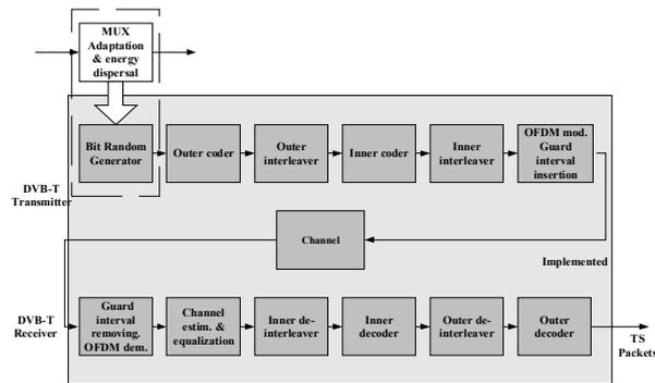
Figure 3. Block diagram of the DVB-T modulator, channel and demodulator.
