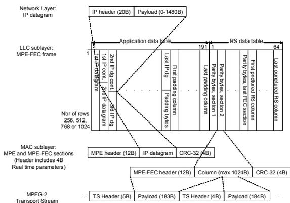
Figure 2. The link layer packets of DVB-H
