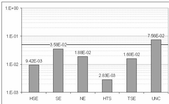
Figure 8. Ratio of visible erroneous seconds,  $C/N = 14$  dB,  $f_D = 10$  Hz (MFER SE  $\approx 5\%$ ).
