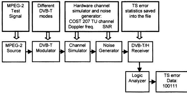
Figure 5. Measurement setup for obtaining TS packet error traces
