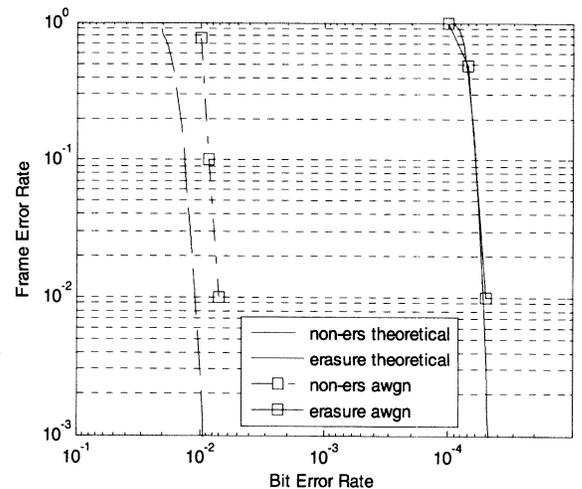
Figure 4. Theoretical versus AWGN simulations
