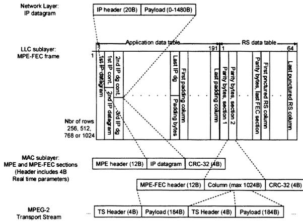
Figure 2. The link layer packets of DVB-H
