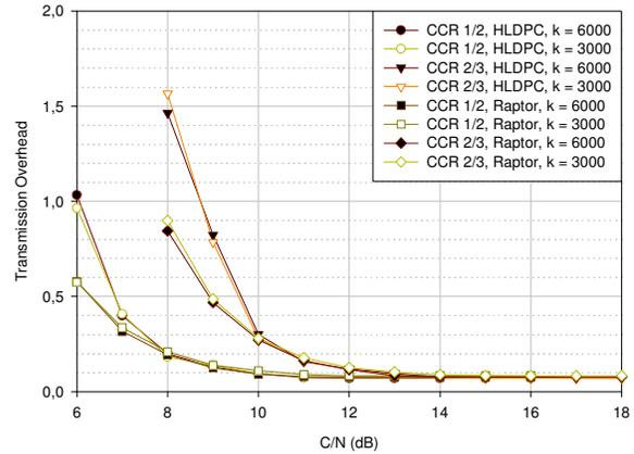
**Fig. 10.** Transmission overheads for HLDPC and Raptor codes on a QPSK-modulated TU6 channel with convolutional code rates 1/2 and 2/3.
