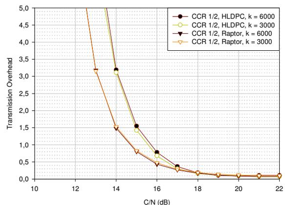
**Fig. 12.** Transmission overheads for HLDPC and Raptor codes on a 64QAM-modulated TU6 channel with convolutional code rate 1/2.
