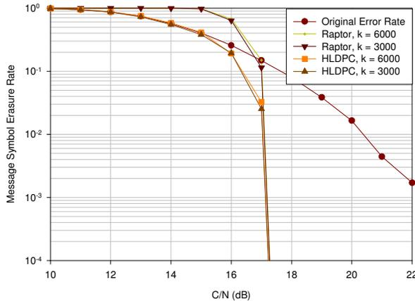
**Fig. 9.** Erasure correction performances of Raptor and HLDPC codes on a 64QAM-modulated TU6 channel with convolutional code rate 1/2.
