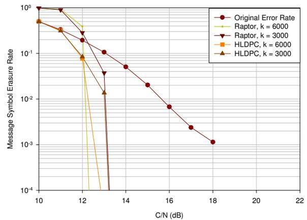
Fig. 7. Erasure correction performances of Raptor and HLDPC codes on a 16QAM-modulated TU6 channel with convolutional code rate  $1/2$ .
