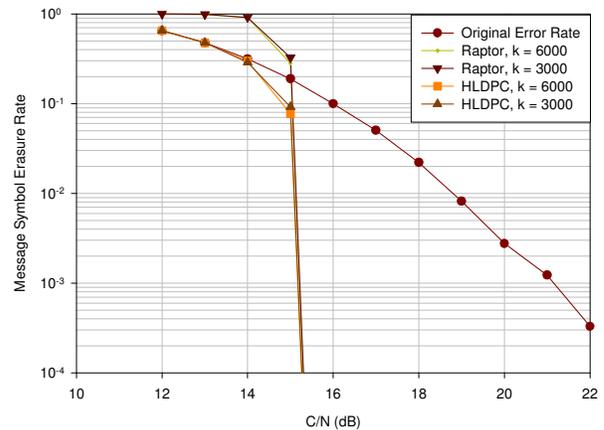
Fig. 8. Erasure correction performances of Raptor and HLDPC codes on a 16QAM-modulated TU6 channel with convolutional code rate  $2/3$ .
