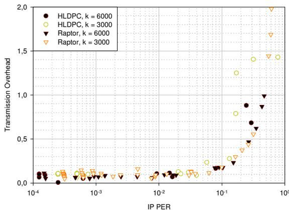
**Fig. 14.** Transmission overhead vs. received IP packet erasure rate for DVB-H mobile pedestrian outdoor measurements using HLDPC and Raptor codes.
