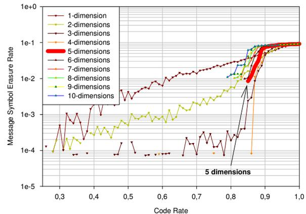
Fig. 4. Message symbol erasure rates vs. code rates for HLDPC codes with 3000 message symbols and up to 10 dimensions on a TU6 channel with Doppler frequency 79 Hz. 5-dimensional codes are the most beneficial ones.
