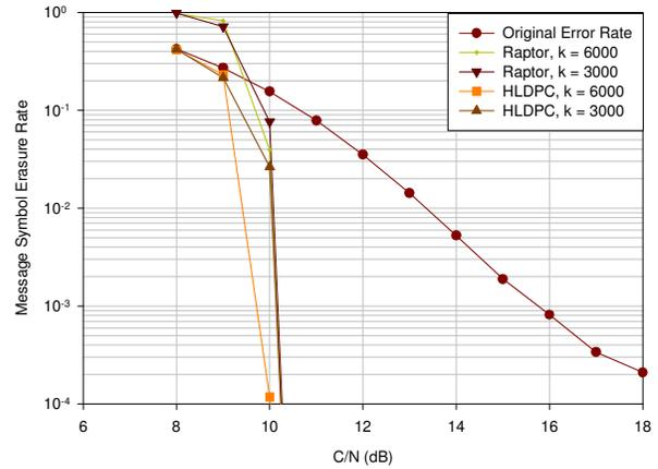
Fig. 6. Erasure correction performances of Raptor and HLDPC codes on a QPSK-modulated TU6 channel with convolutional code rate  $2/3$ .
