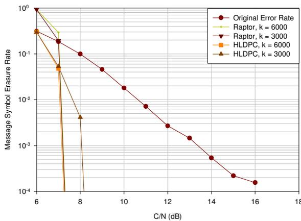
Fig. 5. Erasure correction performances of Raptor and HLDPC codes on a QPSK-modulated TU6 channel with convolutional code rate  $1/2$ .
