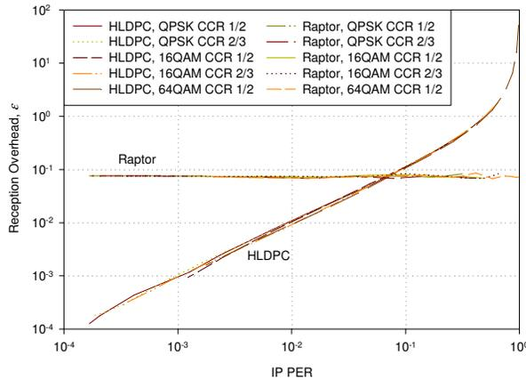
**Fig. 13.** Reception overhead vs. IP packet erasure rate for an interleaved 5-dimensional (8000, 6000) HLDPC code compared to an equal length Raptor code on a QPSK-, 16QAM-, and 64QAM-modulated TU6 channel, with convolutional code rates 1/2 and 2/3.
