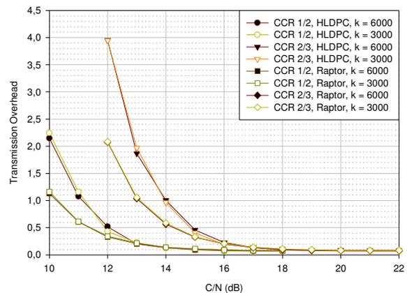
**Fig. 11.** Transmission overheads for HLDPC and Raptor codes on a 16QAM-modulated TU6 channel with convolutional code rates 1/2 and 2/3.
