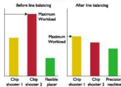
Figure 5. In intraline balancing, the optimization criterion is minimizing a machine's workload within the maximum workload.
