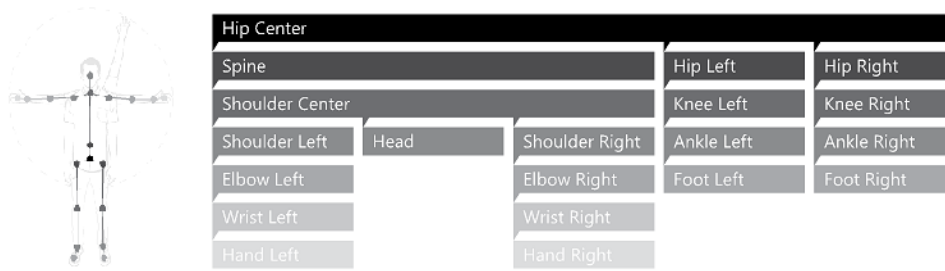
Figure 4.7: Left: Skeleton, bones and joints. Right: Joints hierarchy. [Kinect for Windows]
