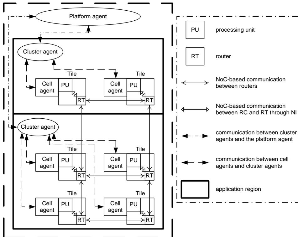
Figure 2: A many-core platform architecture with hierarchical agents
