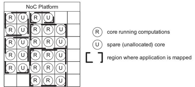
Fig. 4. Application mapping.
