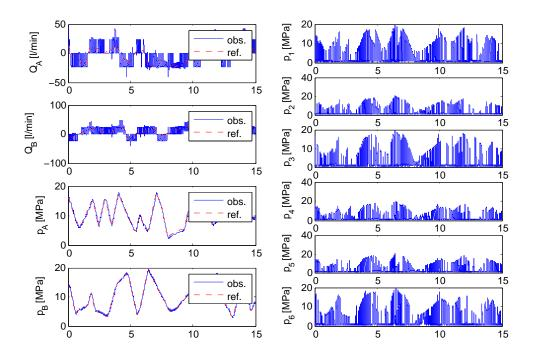
Figure 2: Results from a simulation of System 1. The figures to the left show flows Q and pressures p in the A and B-lines. The figures to the right shows pressures in the pumping cylinders 1..6.
