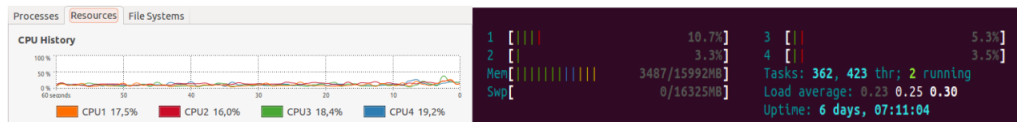
Figure 14: Load calculated as a busy vs. idle time ratio presented in system monitor and htop
